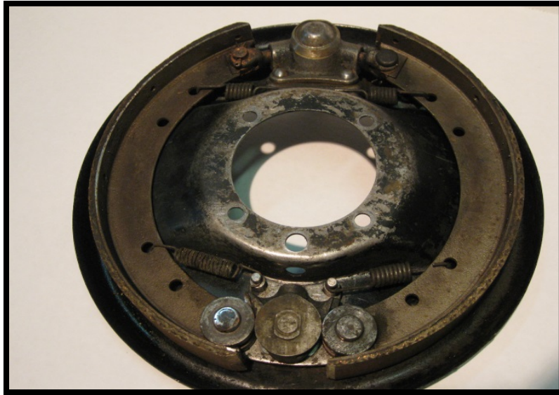
Fig 1 - Brake pins installed incorrectly
