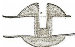
Fig. 3 Appearance after drilling
