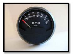
The tachometer face is shown on the left. It is a simple unit to wire up, on the back there are two pins, #2 and #5. You connect a wire from pin #2 to the passenger side of the coil and a wire from pin #5 to the driver's side of the coil. If you buy a light kit you will have to decide how to wire it. On my car I ran a wire from the light to ground and the other wire to my water temperature gauge's light. If you are
