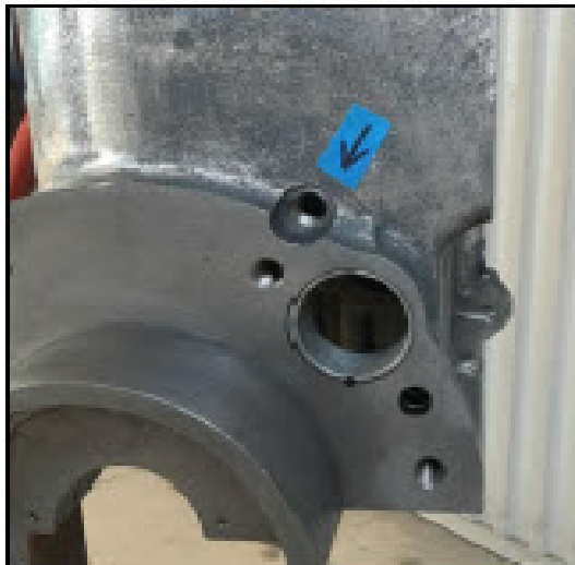
The arrow shows where a 1/2 inch long, 1/2-13 socket head cap screw (Allen screw) with an aluminum sealing washer was installed.
