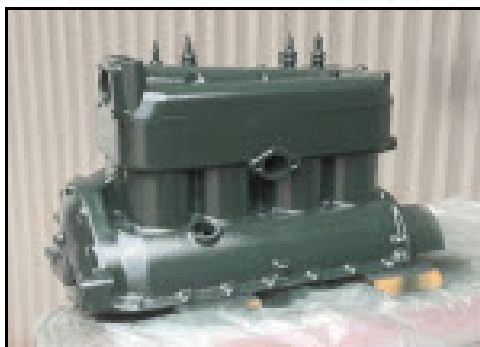
The head, block and front cover are temporarily installed for painting.
