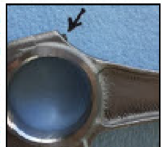
Arrow indicates where rod cap bolt protruded slightly.
