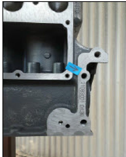
The arrow points to an oil passage hole that must be plugged and sealed by a 7/16-14 "set screw".
