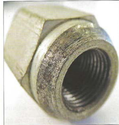
Above - lug nut with full threads
