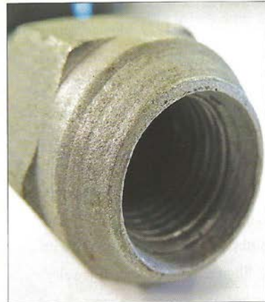
Above - lug nut with relieved threads
