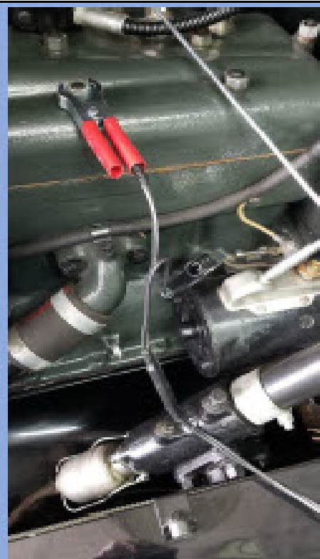
Red clip is ground, black is power No need to connect directly to car battery
