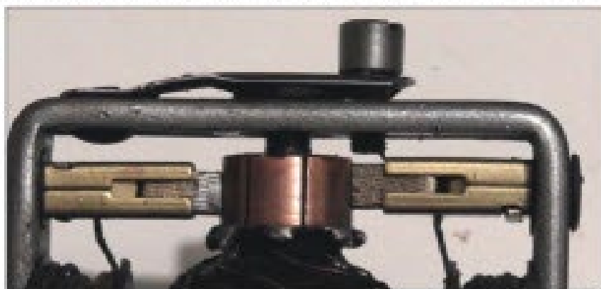
Photo 2: The armature has worn short.
