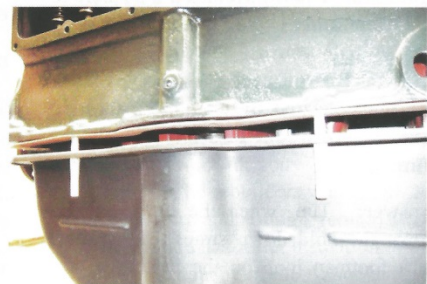
Photo 3 The pan is also held in position by the Snapups.
