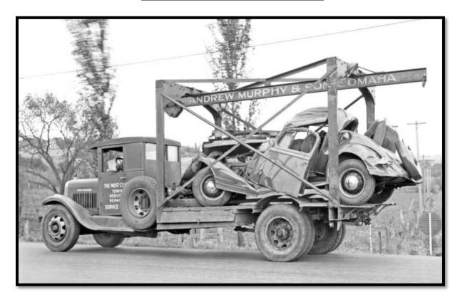
One look at this truck with a wrecked mid-1930s coupe on board told us that this wasn't your run of the mill International tow truck used for bringing in inoperable or crashed cars. After some thought, it appears that this machine may have been an old rigger's truck pressed into service by Andrew Murphy & Sons of Omaha, NB, for picking up and transporting damaged cars.
