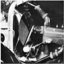
The "powerhouse" generator, which is considered by some as a trademark of the 1928's, actually appeared in three different forms. The very early A's had a cadmium plated adjusting arm which held the generator in Position. The cutout was located on the side of this powerhouse generator. The most significant difference, however, was the finish of the back or end cover on the generator. The end cover was either unpainted aluminum or metal plated with dull nickel or cadmium, again unpainted.
