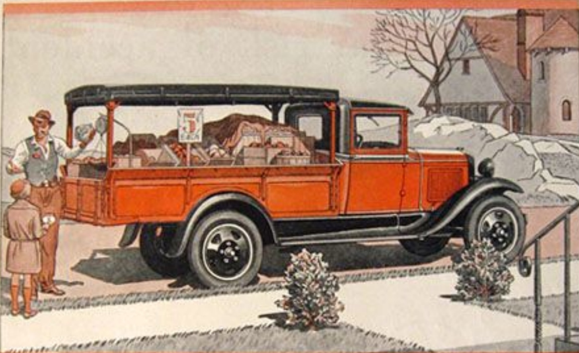
The Light-express Body equipped with Canopy Top. A type widely used by bookstores, vendors, grocers and others, for newspapers and magazine deliveries, and for many other purposes. Made of steel, except for floor-boards and sills, which are of specially annealed wood. The steel end-gate is equipped with heavy chains. Screen tubes can be supplied.
