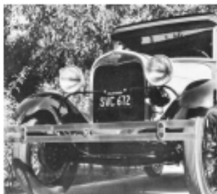
Bumper with flat rounded, open end, without the usual bolt, is one of the more obvious features of a true "early bird." Also notice round center bumper clamp with Ford script and "made in USA" - same as Model T
